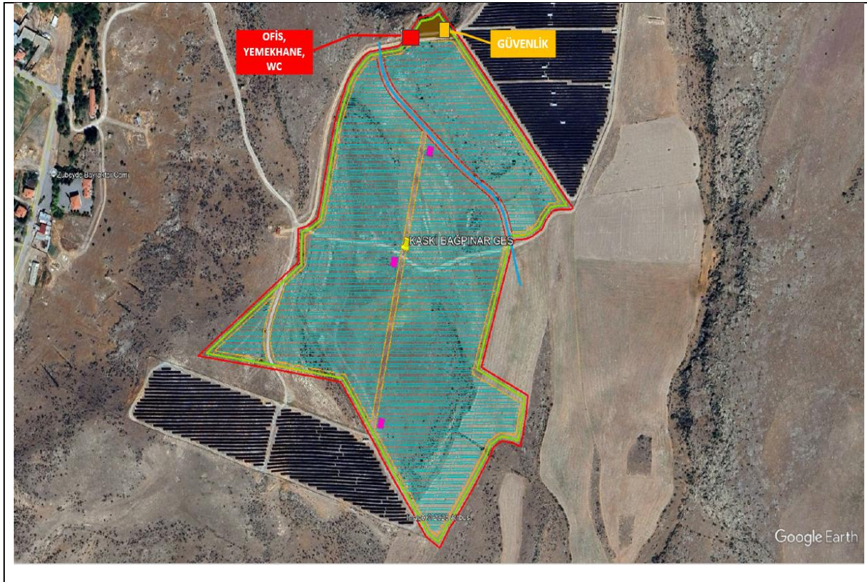
Figure 14. Construction Camp Site Layout
